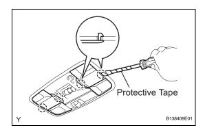
(b) Using a screwdriver with its tip wrapped in protective tape, disengage the 2 claws and remove the cover.
