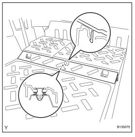
(b) Disengage the clip and the claw and remove the rear floor board.
