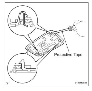
(c) Using a screwdriver with its tip wrapped in protective tape, disengage the 4 claws and remove the room light.
