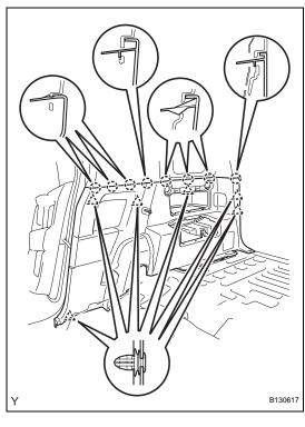
(b) Disengage the 6 clips and the 8 claws and remove the deck trim side panel.
