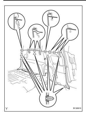
(b) Disengage the 6 clips and the 8 claws and remove the deck trim side panel.
