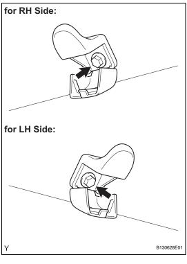
(b) Remove the bolt and the coat hook.
