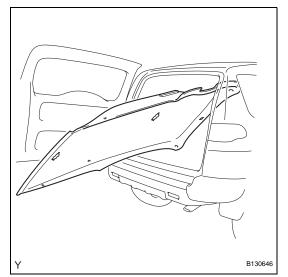
(f) Remove the roof headlining from the back door.
