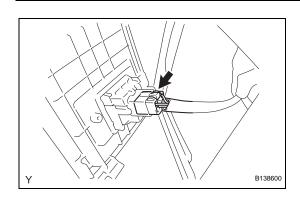
(b) Disconnect the power outlet connector.
