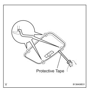
(a) Using a screwdriver with its tip wrapped in protective tape, disengage the 4 claws and remove the room light lens.
